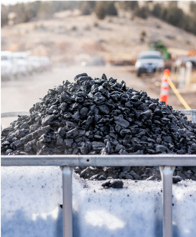
Biochar stormwater filtration media. Photo by Marcus Kaufmann, Oregon Department of Forestry
